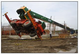
November 09, 2004, Pedestal Crane Floating Articulation Boom with capacity 8 Ton mounted/install on MV. Qal Ranger, "COLLAPS" during lifting food basket 1, 5 Ton in Total E&P Indonesie at plat form MWP – C Peciko sites.
