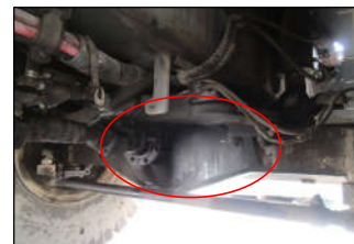
Fig. 9) View of leak on rear axle crane AZ 309841
