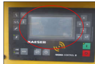
Fig. 7-8) View of blurry control interface on screw compressor
