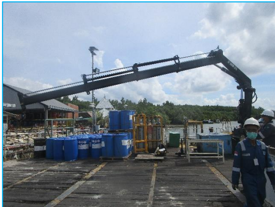
View of Function and Performance Test 15% SWL
