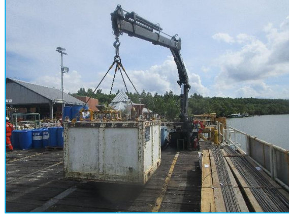
View of Function and Performance Test 15% SWL
