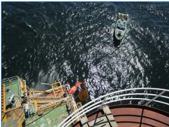
SWL 3 Ton @ Dynamic Load 1 Partline
