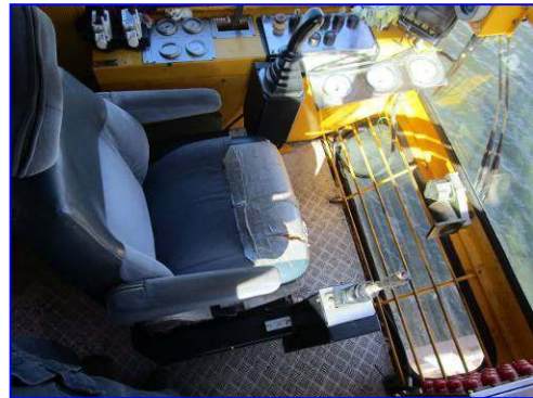
Operator leather seat was broken, should be repaired
