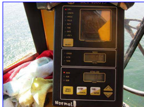
Load Indicator RCI – 4000 /S ROBWAY S/N 0281 Boom Angle Degree Display Malfunction
